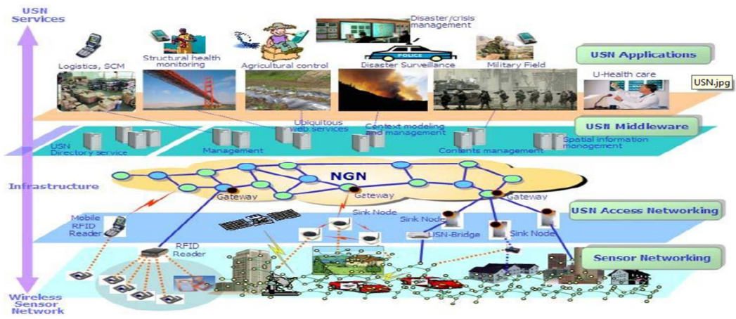
Figure 6. NGN based wireless sensor networks
